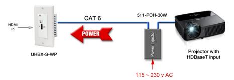
The inserter has a universal AC input and can be connected to 100~230 VAC. The package and includes North American Power cord (customer must provide their own AC input cables when used with other standards).
