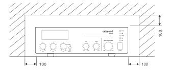
Keep the unit's all sides over 10 cm away from objects that may obstruct air flow to prevent the unit's internal temperature rise.
