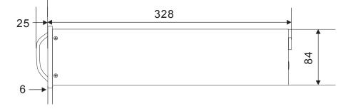
Keep the unit's all sides over 10 cm away from objects that may obstruct air flow to prevent the unit's internal temperature rise.
