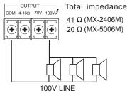
• During installation of the speakers, make sure the sum of nominal input power of the speakers to be connected is lower than the nominal power of the equipment.
