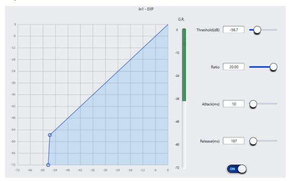
**Threshold:** The expander engages the signal when the signal falls below the threshold value.
