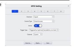
channel when the voltage is below the threshold and automatically unmute when the voltage is above the threshold. "Triggered by high level (Cancelled by low level)" will trigger the channel when the voltage is above the threshold and automatically unmute when the voltage is below the threshold.
