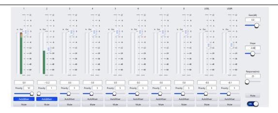
**Gain(db):** Determines the desired target gain for the output of the automixer module.
