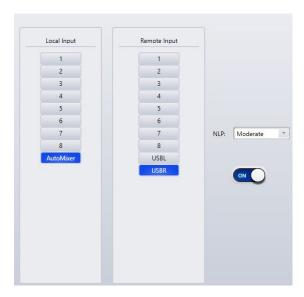
**Local Input:** Selects the audio source or sources that contains the desired audio signal as well as unwanted echoes from the remote signal.
