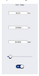
**Milliseconds, Meters and Feet:** These parameters are interlinked, the display the same delay time measured in three distinct units. Adjusting a value in any one of the parameters will automatically be converted to the other units of measure and filled in.
