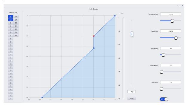
**Reference Source:** Sets the reference channel to trigger the Ducker to engage. More than one channel can be selected as reference sources.
