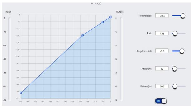
**Threshold:** When the audio signal level is below the threshold, the input-to-output ratio is 1:1. If the signal level is above the threshold level, the input-to-output ratio changes according to the assigned ratio value.
