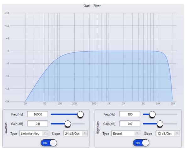
**Frequency(Hz):** Sets the cutoff frequency of each filter. The cutoff frequency of Bessel and Butterworth are selectable in -3 dB steps, and the cutoff frequency of Linkwitz-Riley are selectable in -6dB steps.
