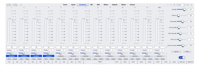
**Gain(dB):** Determines the desired target gain for the output of the automixer module.
