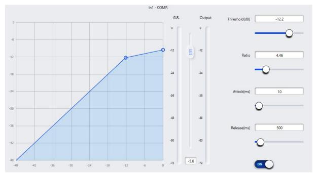
**Threshold:** If a signal crosses above the threshold of the compressor the compressor will be engaged.
