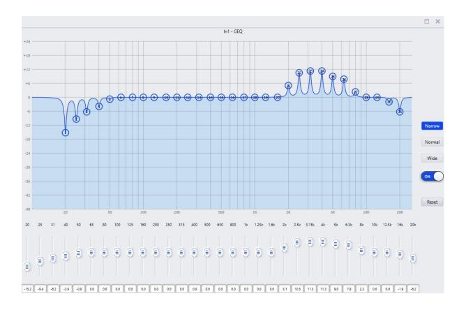
**Frequency Bands:** Gain control for the specified frequency. The value range is between +12 dB and -24 dB (attenuation).
