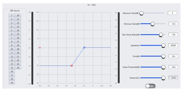
**Reference Source:** Sets the reference channel where the "listening" microphone is connected. More than one channel can be selected as reference sources in a large space.
