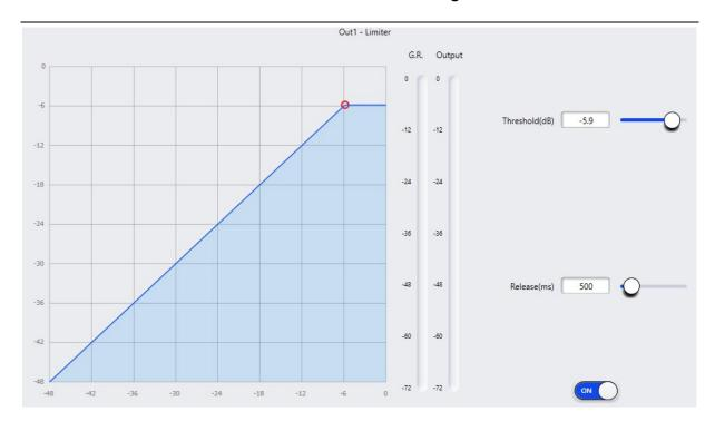
**Threshold(db):** If a signal pass above the set threshold the Limiter will be engaged.
