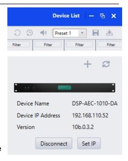
The following shows the Home Tab view of the interface (using Light Mode theme). Use button and select model to add multiple DSPs to control simultaneously.
