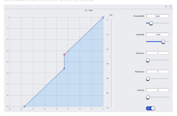
**Threshold(dB):** Audio signals above the set threshold passes, and audio signals below the threshold are attenuated.
