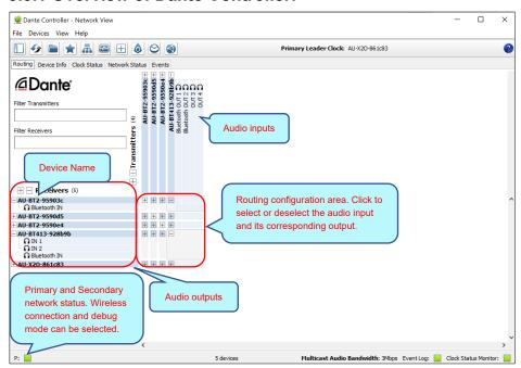
The default setting only supports 2 transmit and 2 receive flows in unicast mode, if more than 2 transmitt streams are needed multicast must be configured.
