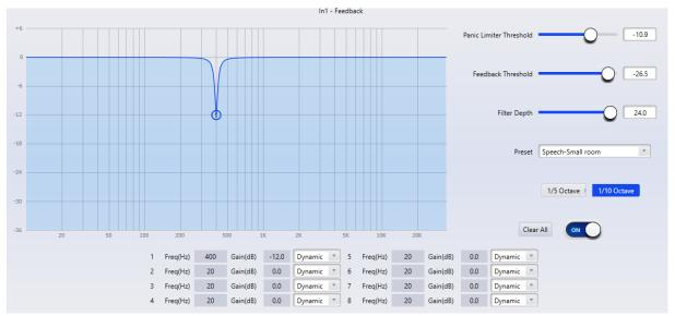
**Panic Threshold:** Any signal crossing above the Panic Threshold will be detected as feedback. When a signal crosses above any of the following will occur to attenuate the feedback:
