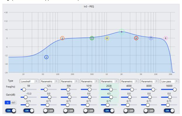
**Frequency (Hz):** Determines the center frequency of the filter.
