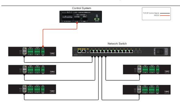
Note: Baudrate for RS232 and RS485 is set globally by software in "Device Settings".
