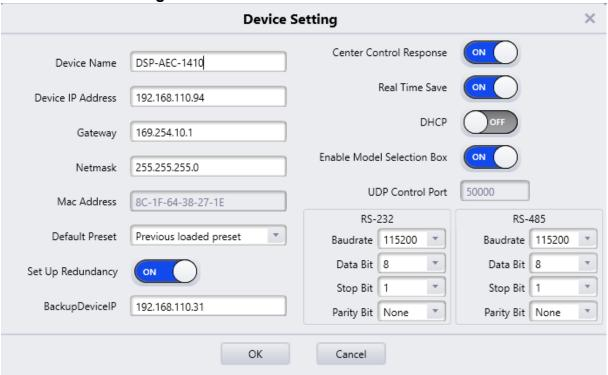
**Device Name:** Set the name of the device and the name will display anywhere the device is addressed. The name is saved into the hardware.
