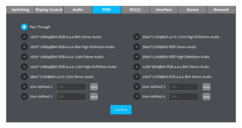
**Note:** Before select EDID in this tab, please ensure the 4-pin DIP switch on the rear panel is on the "1111" position.
