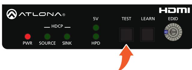
4. The **SOURCE**, **SINK**, **5V**, and **HPD** indicators will display the current testing results. Refer to the table, below.
