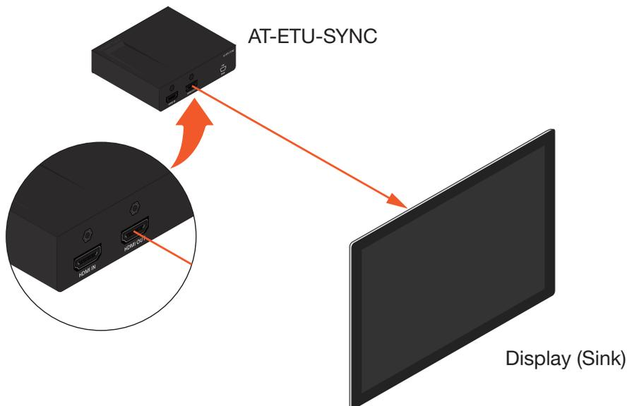
5. Press and hold the **LEARN** button on the AT-ETU-SYNC until the **HPD** light glows green.
