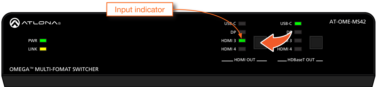
Figure 1.1 - HDMI 3 is selected as the active video input and Laptop 1 has access to the speaker/mic and the AT-HDVS-CAM. Black signal lines indicate that the AT-OME-MS42 is not switched to that input.
