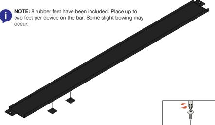
8. \*Optional\* Once the feet are attached, reattach the stabilizing bar to the rack shelf with the previously removed screw and washer.
