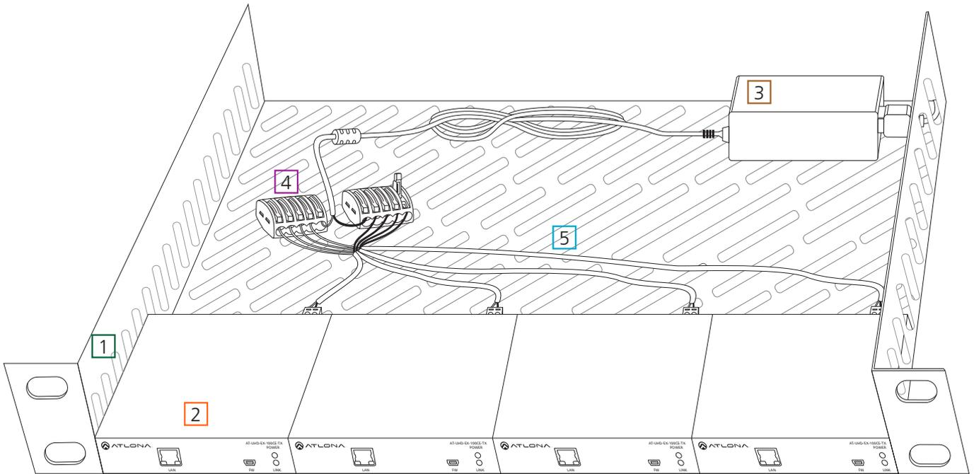
To chain one power supply to three transmitters (four when using AT-PSU-48V1.25A), use two wago splicing connectors, 18/2 AWG stranded wire, a ventilated 1 RU rack shelf, zip ties, and high temperature hook and loop (velcro) strips will be needed.
