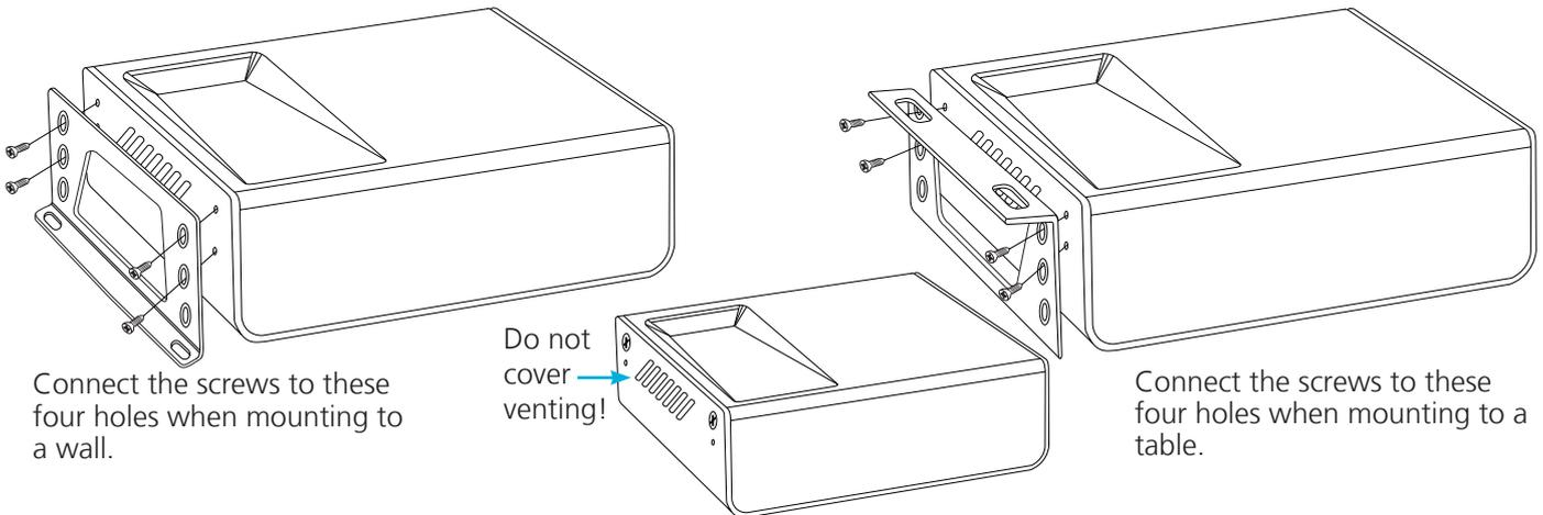
Connect the screws to these four holes when mounting to a wall.
