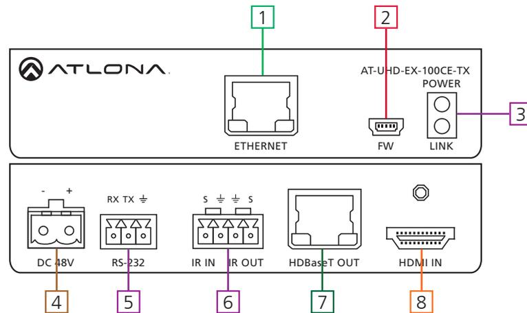
1. **Ethernet** - Connect to a router to send Ethernet signals
