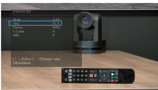
Figure 26: Exposure AAE with Iris F1.8 (left) and F5.6 (right)
