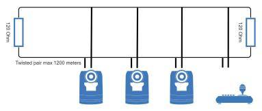
Figure 14: RS-485 Network Connection Diagram
