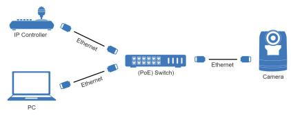
Figure 15: IP Network Connection Diagram
