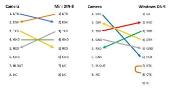
Figure 7: RS-232 Cable and Interface Connection (Mini DIN-8 and Windows DB-9)
