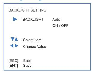
The backlight setting will lighten the buttons of the CON100 to make the buttons visible in dark environments.
