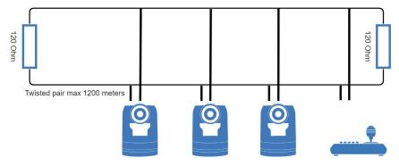
Figure 10: RS-485 Network Connection Diagram
