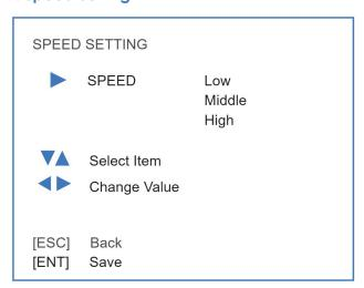
Speed Setting sets the speed to which the camera will respond when you move the camera by using the joystick.
