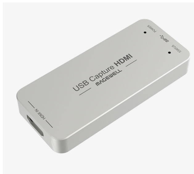
Figure H.1 - Magewell USB Capture HDMI Gen 2
