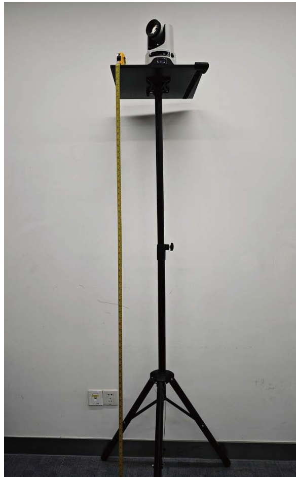
Figure 4. Camera installation height
