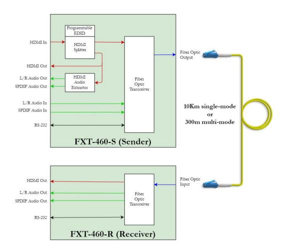
The FXT-460-S Sender provides a HDMI input with a corresponding HDMI loop output. The audio component of the HDMI input is extracted and available as both analog (L/R) and Digital SPDIF (TOSLINK) on corresponding connectors (see diagram above).
