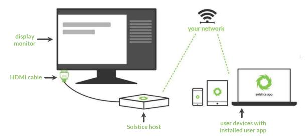
The requirements for an operational Solstice system are straightforward. The Solstice Pod or Solstice Windows host PC is directly connected to a display monitor via HDMI cable. The Solstice host is attached to the WiFi/Ethernet network that participants will use to connect and share to the display. Then, users on the network can follow the on-screen instructions to get the Solstice app and connect to the display.
