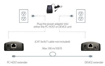
Note: Flexible power is different from Power over Ethernet (PoE). Ensure that the CAT 5e/6/7 cable is only connected between the PC HOST and DEVICE extenders.
