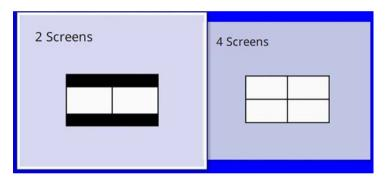
When splitting screen into halves, the currently selected input source moves to the left of the screen.
