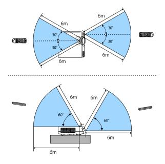
Avoid using the remote control in conditions with bright fluorescent lights or in direct sunlight, or the projector may not respond to commands. If you are not going to use the remote control for a long time, remove the batteries.
