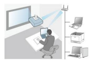
Your projector has built-in wireless LAN modules. If you install an additional optional wireless LAN module, you can use both network connection methods at the same time. When you install the wireless LAN module, set the **Simple AP** setting to **On**.
