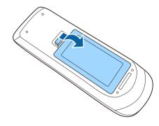
Remove the old batteries, if necessary.
