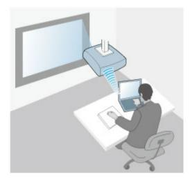
• Infrastructure mode lets you connect to smartphones, tablets, or computers over a wireless network access point. When you use this method, connect the projector using **Advanced Connection Mode** of the Epson iProjection software.
