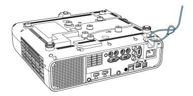
When installing the cable cover (EB-L265F)
