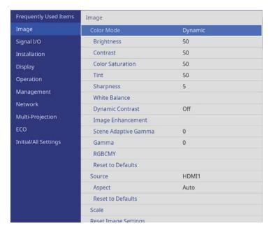
Press the up or down arrow buttons to move through the menus listed on the left. The settings for each menu are displayed on the right.
