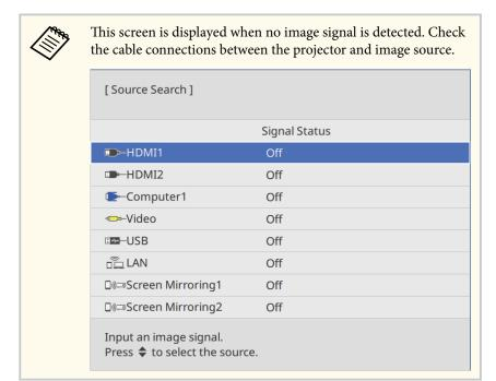
• Press the button for the source you want on the remote control. If there is more than one port for that source, press the button again to cycle through the sources.
