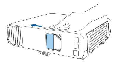
To cover the lens or temporarily turn off the projected image and sound, close the lens cover.
