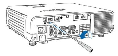
Connect the wireless LAN module to the USB-A port.
